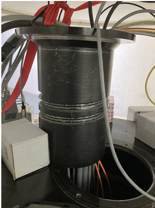
Fig. 3: Spiral track in the central tube, which translates the rotary movement to the sliding motion.
