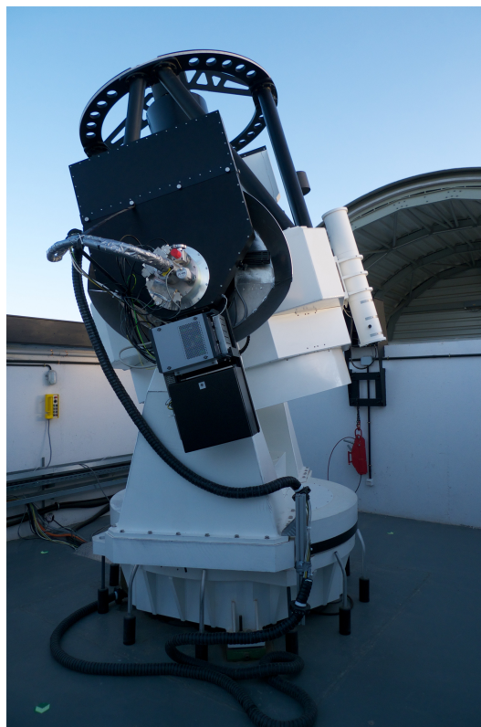
Fig. 1: The STELLA-I telescope during operation with the WiFSIP instrument in front.
