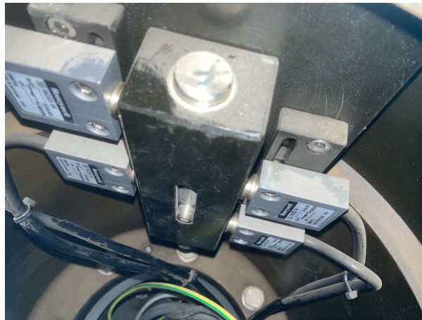
Fig. 2: Vertical slider which triggers the azimuth limit switches.
